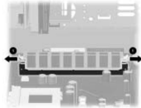
opening the latches on the memory module socket
